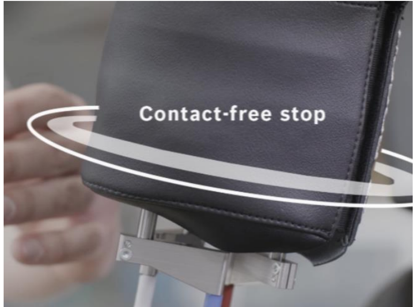
Sensor skin and the shut-off distance around it.
