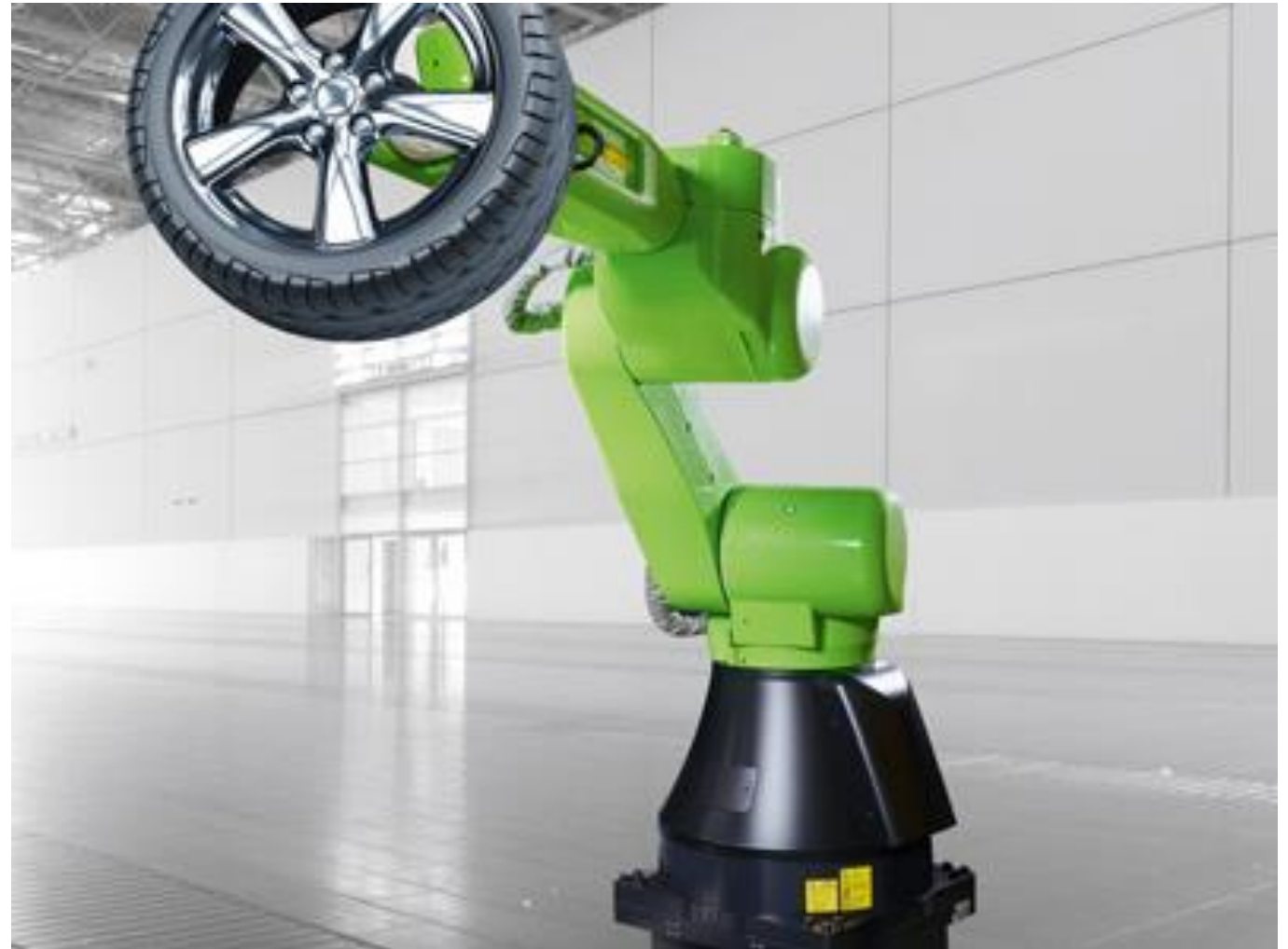
CR-35iA demonstrating its lifting capacity
